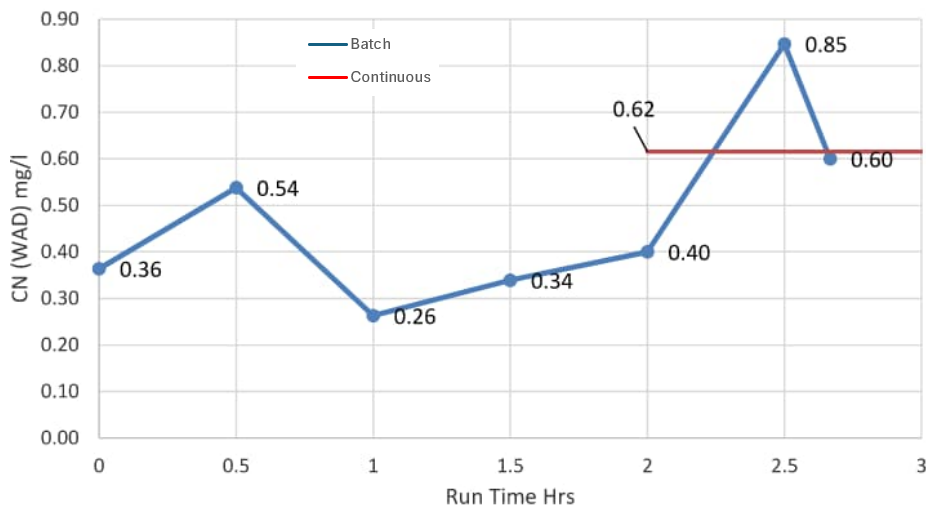
Figure 13-9 – Results of SO 2 Air Cyanide Destruction Testing – Continuous
